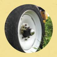
Drive Wheel Disengagement Lock-out hub disengages driveshaft during transport.
