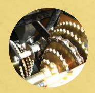
5-Speed Derailleur5-speed derailleur controlsoutput from the fluffy seed box.
